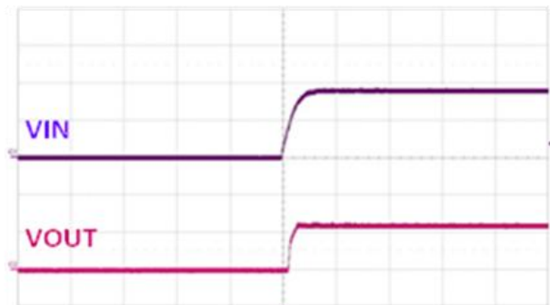
(VIN: 2V/div, VOUT: 2V/div, 1ms/div) Vin=3.5V, Vout=2.5V @ Iout=1A
