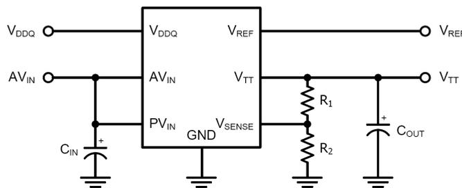
FIGURE 4. Increased VTT from the Scaling Factor
